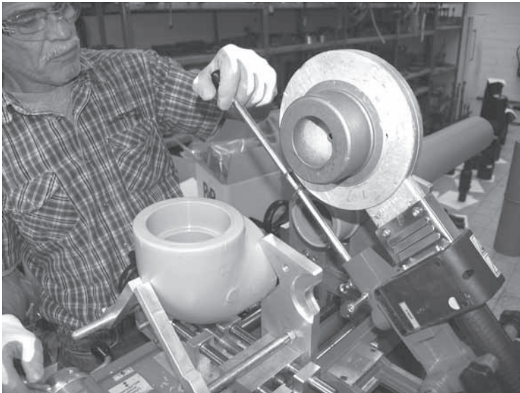
Fig. 4 Move the machine slides with the handle lock to set the heating element into the center between pipe and fitting
