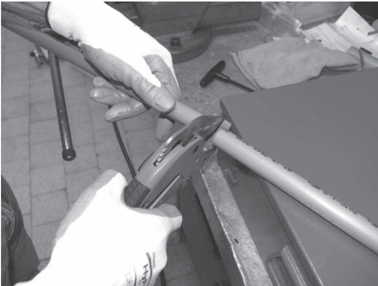
Fig. 1 Cut the pipe perpendicularly with a suitable pipe cutter.
