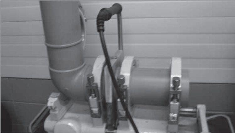
Fig. 3 During butt welding with heating elements the areas to be joined are heated up to the welding temperature by means of the heating element and compressed after the heating element has been removed. Heating temperature 410^{\circ}\text{F} \pm 50^{\circ}\text{F} .
