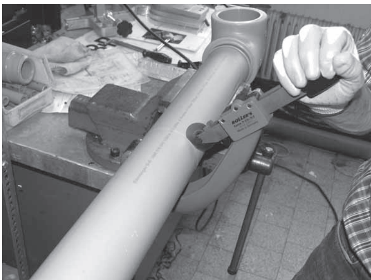
Fig. 1 Pipes are measured and cut with suitable pipe cutters to the required length. Cutting should be perpendicular to the pipe axis (90°).
