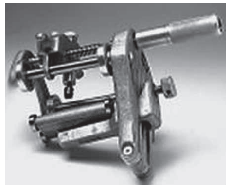
Fig. 3 For dimensions bigger than 3" (O.D.) we recommend using a peeling tool similar to the one shown above for removing the outside oxide layer.
