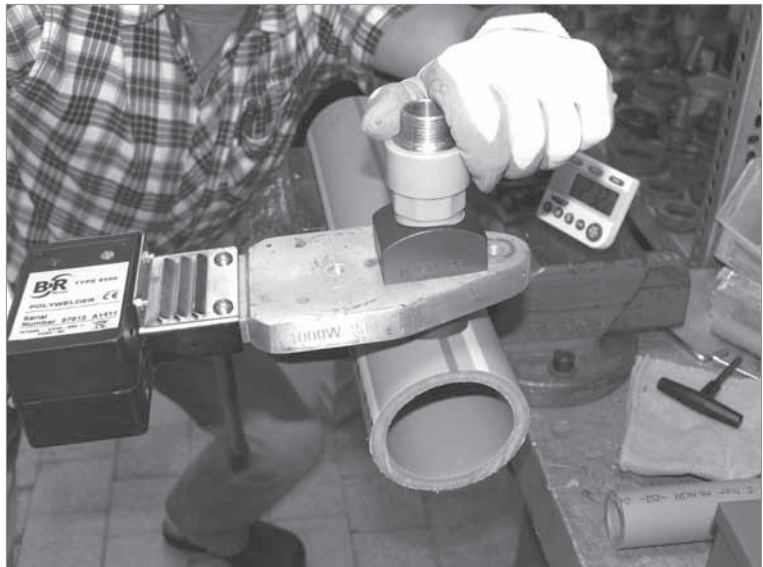
Fig. 2 Push in the heat nozzle of a suitable welding saddle tool in the drill as well as the connecting piece of the welding saddle in the heating socket of a suitable polywelder. The heating time for all dimensions is about 30 seconds.
