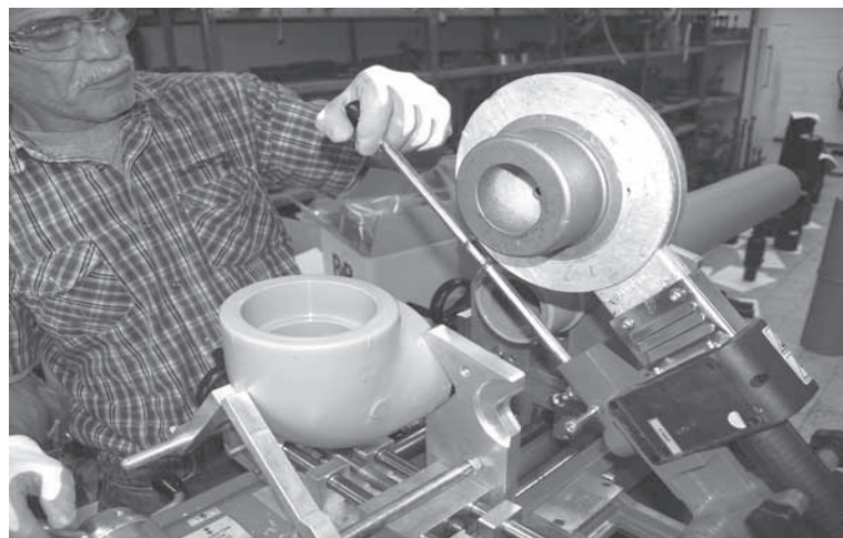
Fig. 6 Move the machine slides with the handle lock and remove the heating element.
