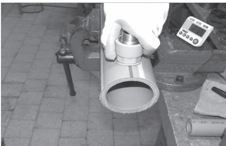
Fig. 3 Push the connecting piece of the welding saddle quickly into the heated bore hole. Push the fitting for about 15 seconds onto the pipe.
