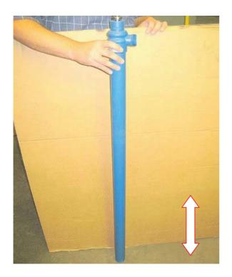
Lightly tap the bottom of the shaft on the ground.
