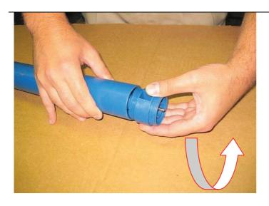
Reinstall the impeller housing cover by turning counterclockwise
