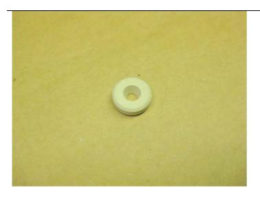
Top view of new seal (tapered side)
