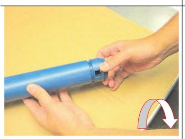
Remove the impeller housing by turning it clockwise.
