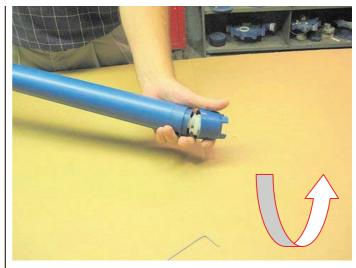
Install impeller housing cover (turn counterclockwise).
