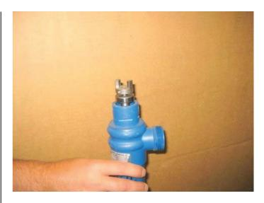
Picture showing bearing assembly partially removed from pump head.
