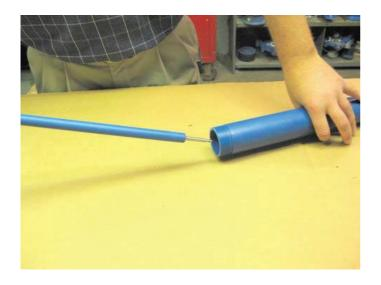
Insert outer tube over shaft assembly.
