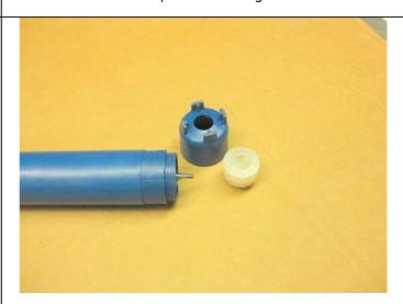
Once the impeller is removed, the bottom portion of the shaft will be exposed.
