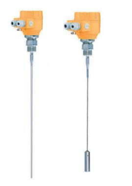
The 2291 Guided Wave Radar level transmitter is designed for continuous level measuring of conductive or non-conductive liquids, pulps and solids. The 2291 level gauge operates based on the well-known TDR (Time Domain Reflectometry) principle. Micropulses are sent along a probe guide at the speed of light. As soon as the impulse reaches the surface of the medium, it is reflected back to the electronic module. Level distance is directly proportional to the flight time of the impulse.
