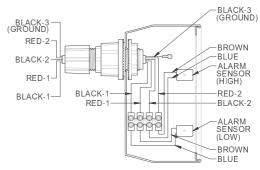
**DUAL ALARM WIRING DIAGRAM**
