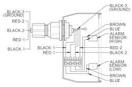
**DUAL ALARM WIRING DIAGRAM**
