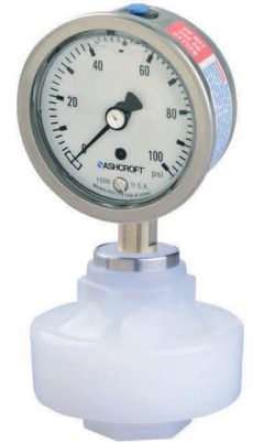
SERIES TG-25SS-PVD 2.5" ALL STAINLESS GAUGE 1/2" Fem NPT Inlet PVDF Body
