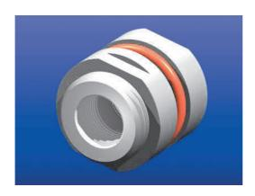
To maximize creep resistance, FLUOR-O-FLO® PTFE bulkhead fittings (and all female FLUOR-O-FLO® fittings) are made from Micromold's MICROFLONTM, a special virgin PTFE. PVDF fittings are made from natural virgin materials. Standard fittings are supplied with Teflon® FEP encapsulated, hollow core, silicone o-rings. PFA encapsulated, or PTFE, or other o-ring materials can be supplied.
