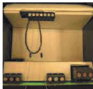
3-Wire RTD Calibration – Precision Resistors and Jumper Wire in Place
