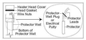
Figure 4 Typical Over Temperature Protector Installation
