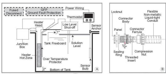
Figure 3 Typical Installation in a Process Tank (A), Flexible Non-Metallic Conduit Connector Installation (B)
