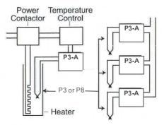
Figure 6 P3/P8 Typical Installation
