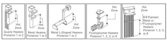
Figure 1 Typical Heaters and their Over Temperature Protectors
