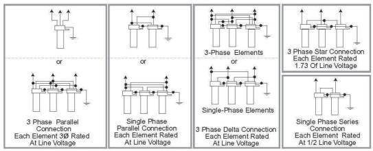
Figure 2 Single and Three Phase Connection Wiring Diagrams
