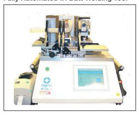
20mm - 110mm (1/2" - 4") Size Range Single wall **Piping** PP, PPn, PVDF, ECTFE **Materials** Plug: 110V Power Tool: 230V / 15A
