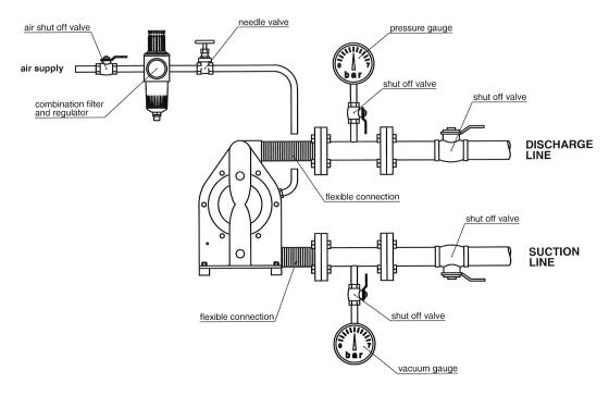
This illustration is a generic representation of a G Series air operated double-diaphragm pump.
