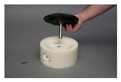
Pull the other diaphragm [14] together with the shaft [13] out of the center block [16].
