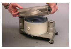
Remove side housing [1] and suction/discharge ports [2].
