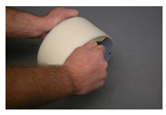
Screw one diaphragm [14] counter clockwise off the shaft [13].
