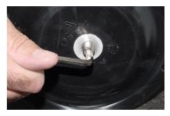
Screw out the set screws, shaft [13a].
